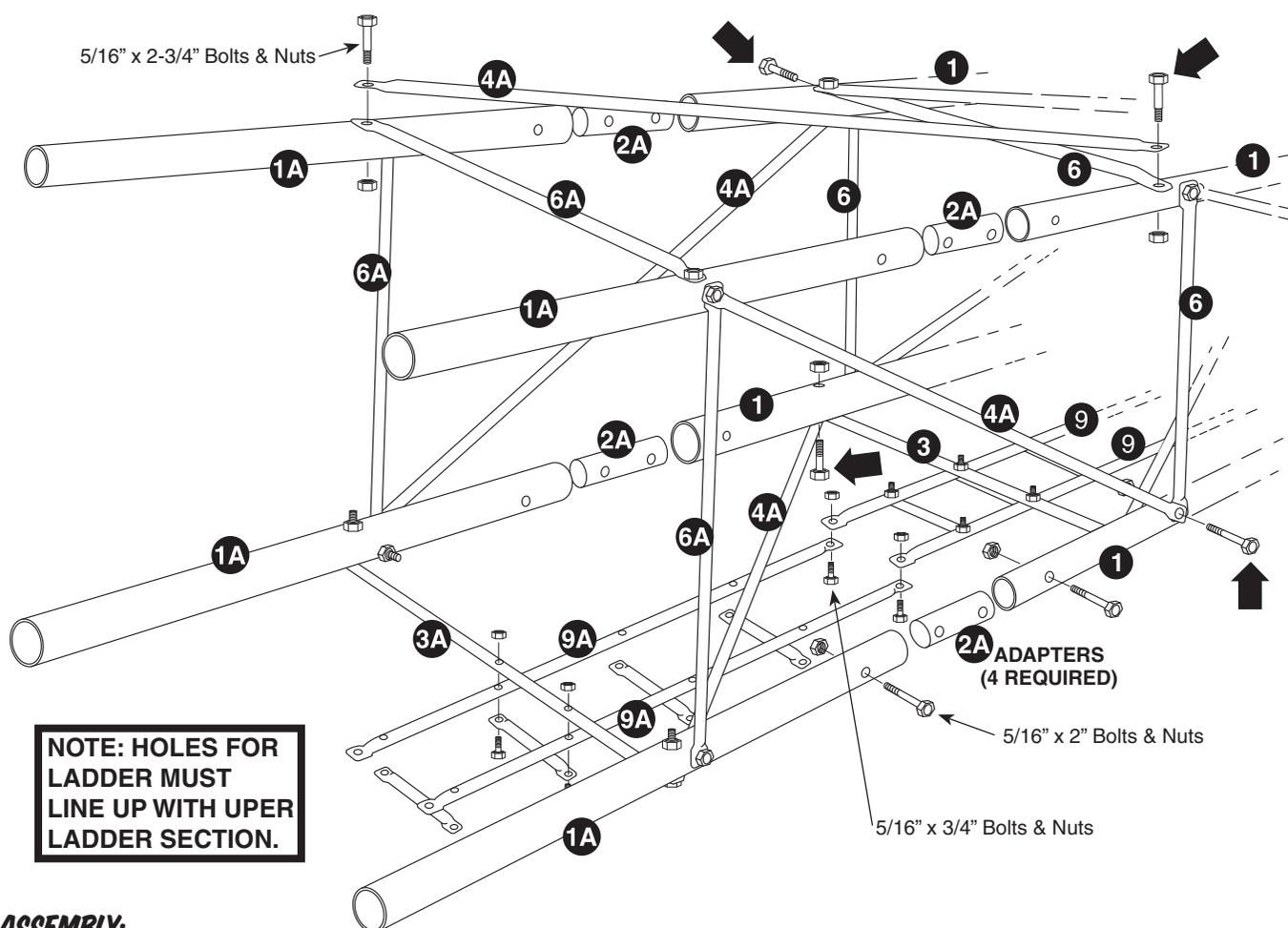
**NOTE: HOLES FOR LADDER MUST LINE UP WITH UPPER LADDER SECTION.**
